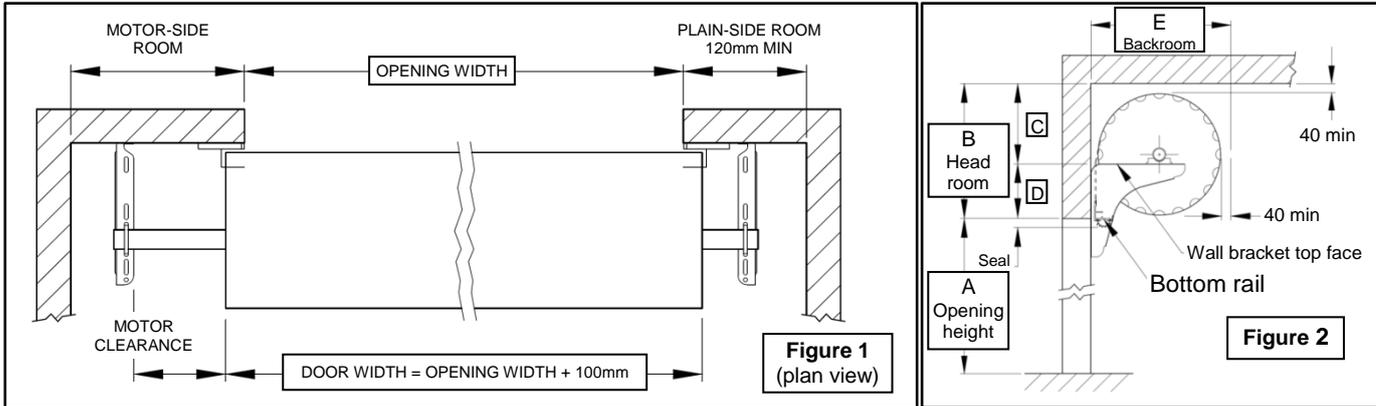
1. Check DOOR WIDTH against OPENING WIDTH (Figure 1). For a standard installation the roller door curtain should be at least 100mm wider overall than the opening.
