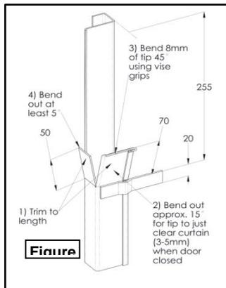
the black plastic button at the end of the Bottom Rail. Ensure the tracks are vertical then fix to the wall by screwing or welding as appropriate.
