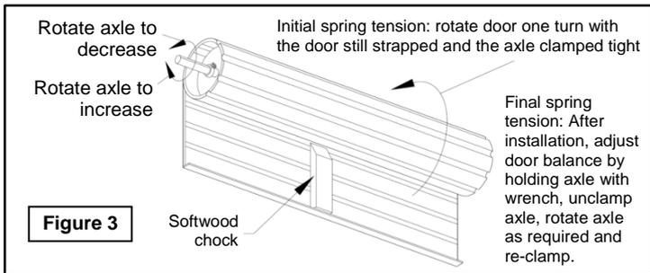
16. Turn the axle to allow the door to be relaxed on the axle with the bottom rail at the bottom of the curtain (6 o'clock position). Hold the door and give the axle a ½ turn of tension (see Figure 3). Fully tighten the axle clamps.
