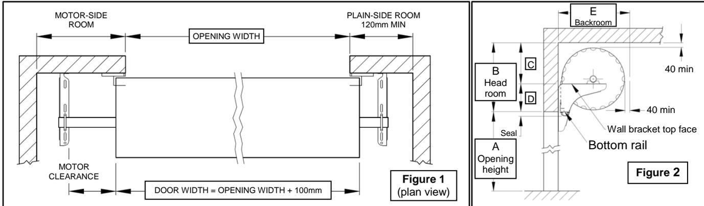
1. Check DOOR WIDTH against OPENING WIDTH (Figure 1). For a standard (non-windlocked) installation the roller door curtain should be at least 100mm wider overall than the opening. For windlocked installation side room increases by 35mm each side. For WINDSTRONG® refer to supplemental instructions.
