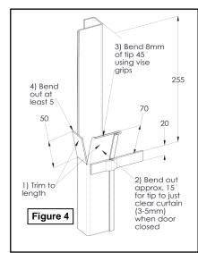
17. Mount the tracks to the wall. Lower the door to the closed position and slide the tracks in from the side until there is a 3-6mm gap between the track and the black plastic button at the
