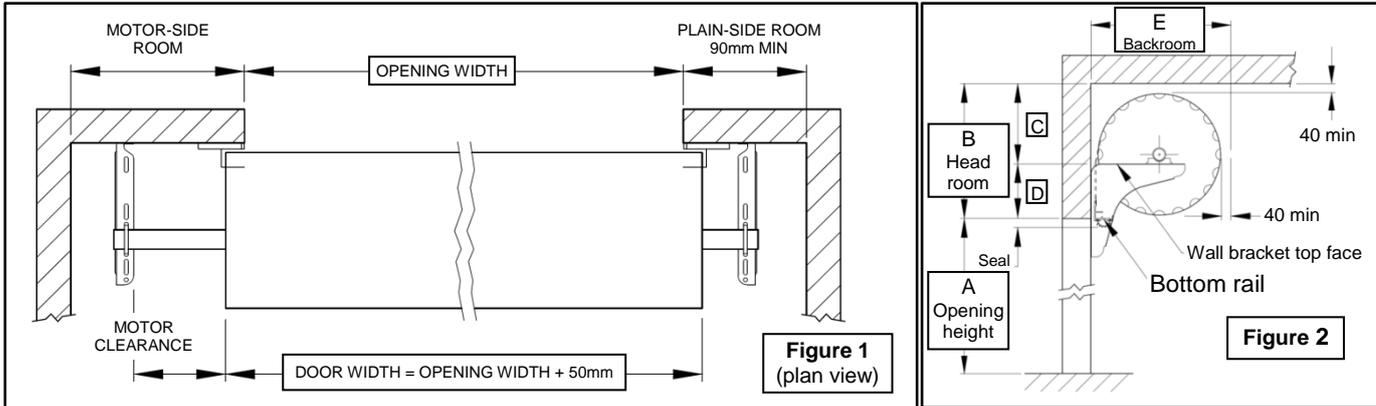
1. Check DOOR WIDTH against OPENING WIDTH (Figure 1). For a standard (non-windlocked) installation the roller door curtain should be at least 50mm wider overall than the opening. For windlocked installation side room increases by 35mm each end and DOOR WIDTH = OW + 100mm. For WINDSTRONG® refer to supplemental instructions.
