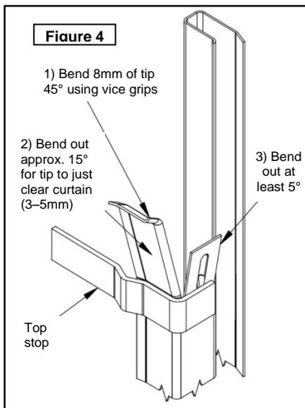
17. Flare out both the side and rear faces at the track lead-in (Figure 4). After fitting the tracks, if necessary adjust the angles so the curtain enters the track smoothly.
