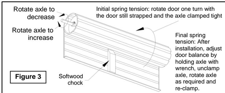
13. Apply 1 turn of spring pre-tension by turning the curtain roll 1 turn over the top and hold in this position (Figure 3).
