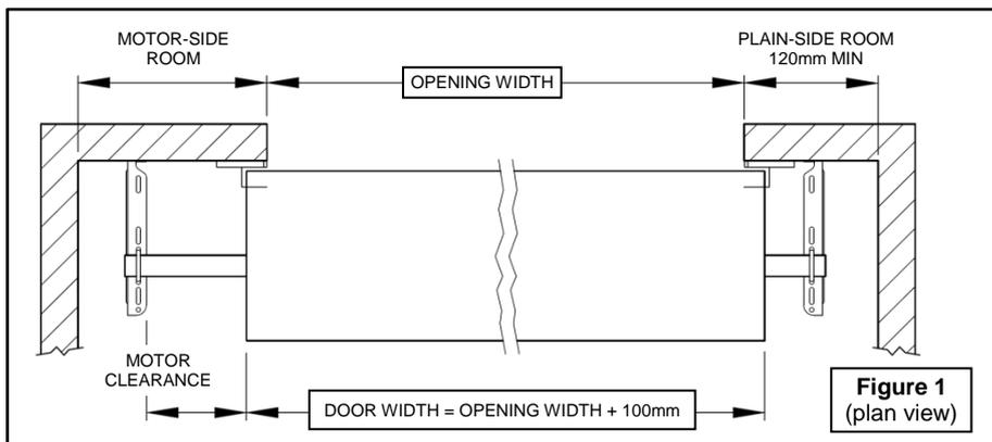
1. Check DOOR WIDTH against OPENING WIDTH (Figure 1). The roller door curtain should be at least 100mm overall wider than the opening.
