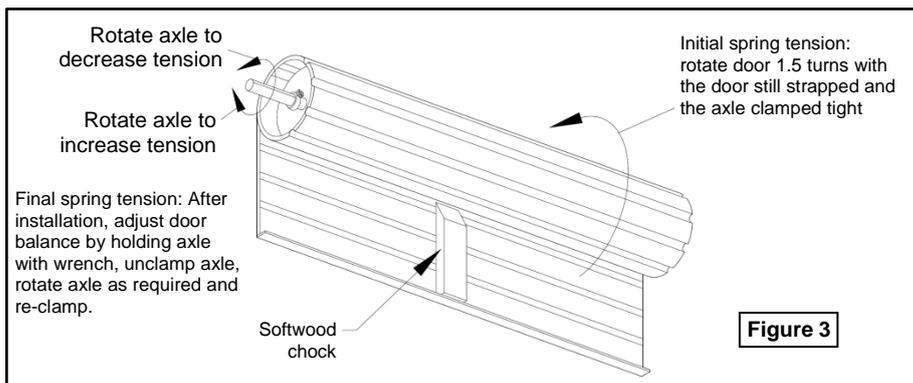
16. Turn the axle to allow the door to be relaxed on the axle with the bottom rail at the bottom of the curtain (6 o'clock position). Hold the door and give the axle a  $\frac{1}{2}$  turn of tension (see Figure 3). Fully tighten the axle clamps.
