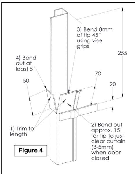
23. **Note:** Before fully fastening the tracks, operate the door fully to ensure it is not binding in the tracks at any point.
